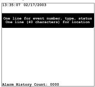
In the center of the 3-LCDXL1 is the Liquid Crystal Display. In the system normal condition the date and time plus a definable system title are displayed on the LCD. The last line of the display gives an alarm history. This total equals the number of times the system has entered the alarm state from the normal state.
